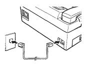
→ Plug one end of the telephone line cord into the TEL LINE jack and the other end into a standard phone jack in your wall.
